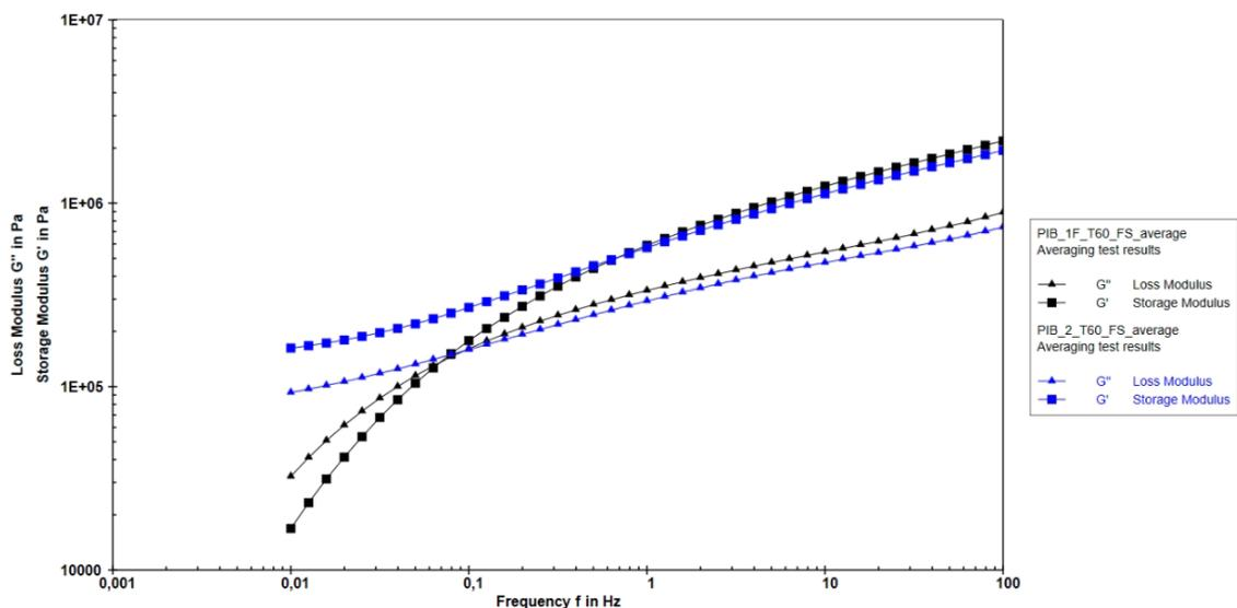
**Figure 4:** Storage  $G'$  and loss  $G''$  modulus as a function of frequency at constant temperature of 60°C (average values are presented).
