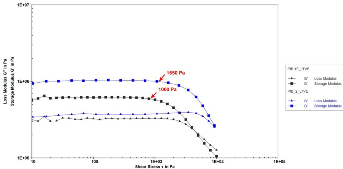
**Figure 3:** Determination of LVTE - storage  $G'$  and loss modulus  $G''$  as a function of shear stress at 60°C.
