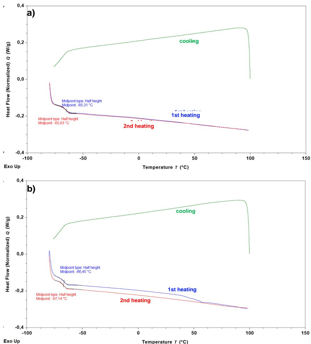
**Figure 2:** DSC thermograms of a) PIB 1 and b) PIB 2 (only 1. repetition is shown).
