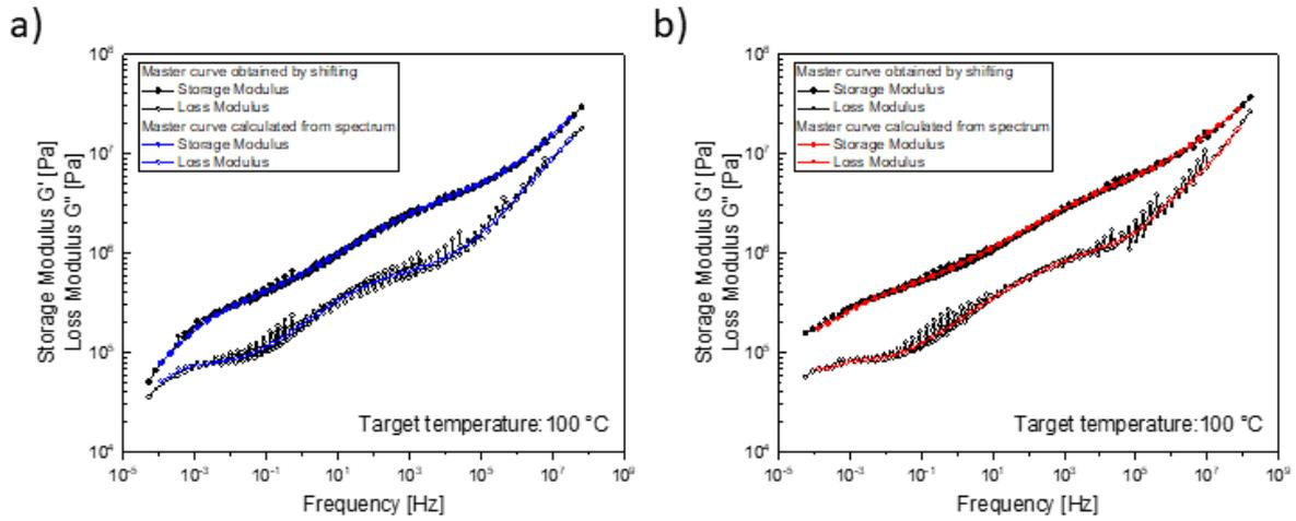
**Figure 4:** Master curves of storage  $G'$  and loss  $G''$  modulus, obtained by shifting isothermal segments (black curve) and calculated from shear relaxation time spectrum (blue/red curve) for a) PIB 1 and b) PIB 2 material.
