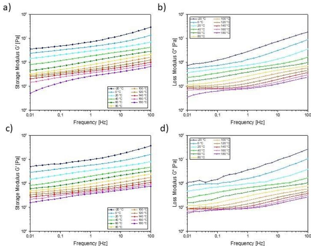
**Figure 2:** Storage  $G'$  and loss  $G''$  modulus as a function of frequency at different temperatures for PIB 1 (a, b) and PIB 2 (c, d) after thermal stabilization (average values are shown).
