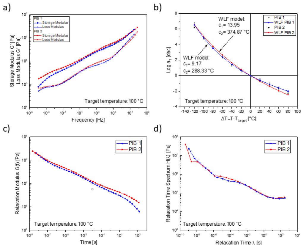
**Figure 3:** a) Master curves of storage  $G'$  and loss  $G''$  modulus, b) horizontal shift factors (WLF included), c) relaxation modulus, d) relaxation time spectrum at target temperature of 20°C for PIB 1 and PIB 2.
