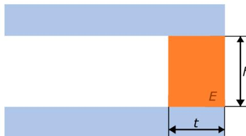
Figure 9: Substitute sealing system model.
