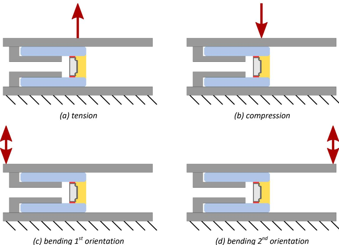
Figure 3: Measurement setups for different load cases.
