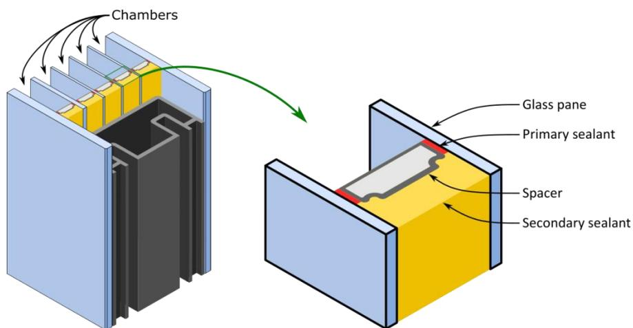
Figure 1: Assembly of a typical sealing system.
