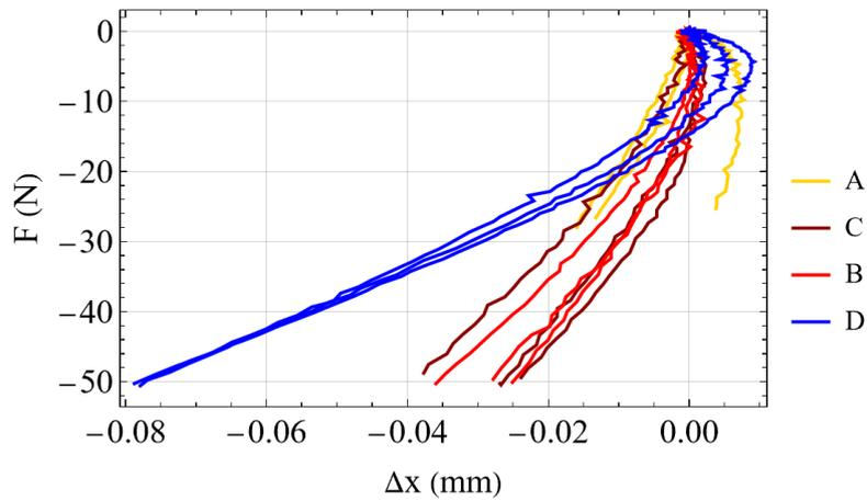
Figure 6: Measured compression response of the sealing system.
