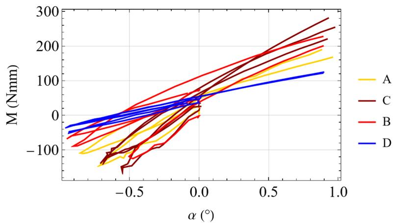
Figure 7: Measured bending response in the 1<sup>st</sup> orientation of the sealing system.
