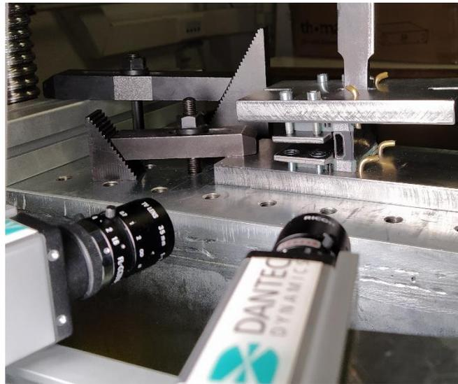
Figure 4: Measurement setup – measurement of the displacements and rotations.
