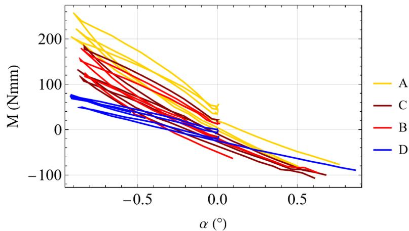
Figure 8: Measured bending response in the 2<sup>nd</sup> orientation of the sealing system.
