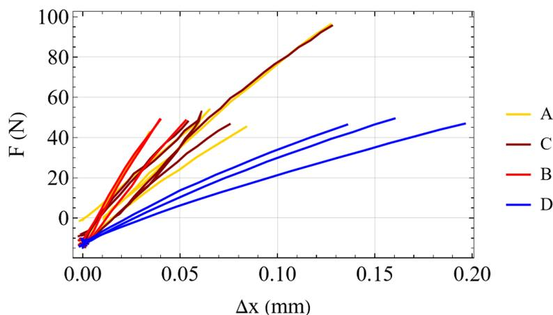
Figure 5: Measured tension response of the sealing system.
