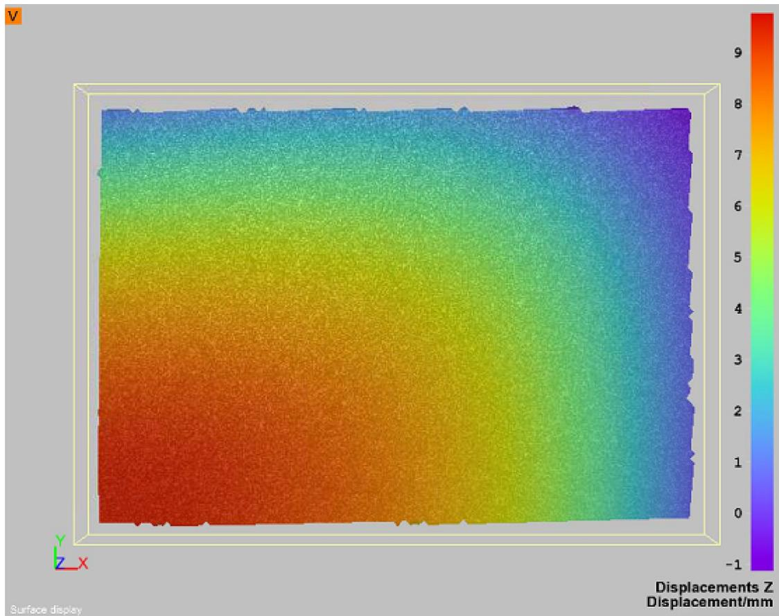
Figure 11: Displacement of sample E at 250 mbar pressure.
