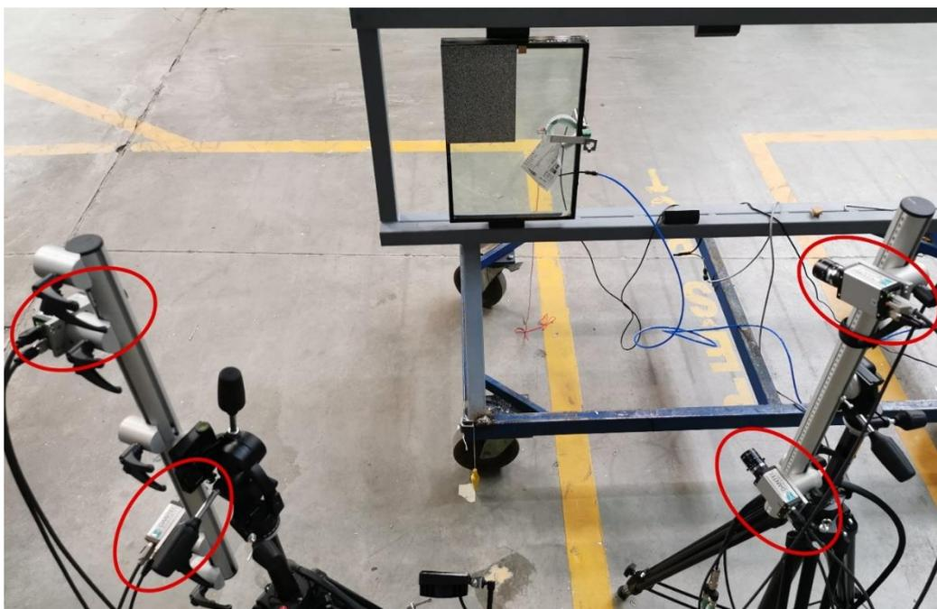
Figure 5: Measurement setup – measurement of displacements of the smallest samples. Cameras are circled in red.
