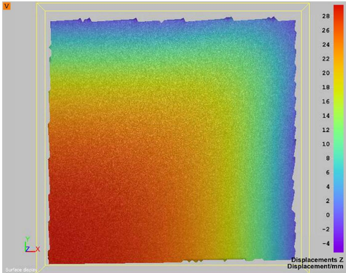
Figure 8: Displacement of sample B at 100 mbar pressure.
