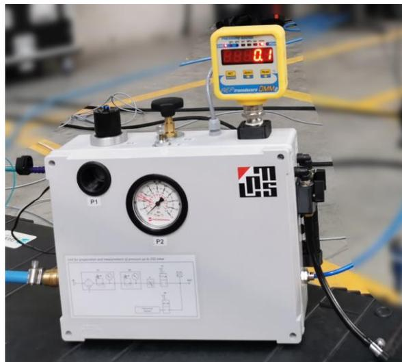
Figure 3: Measurement setup – pressure control and measurement unit.
