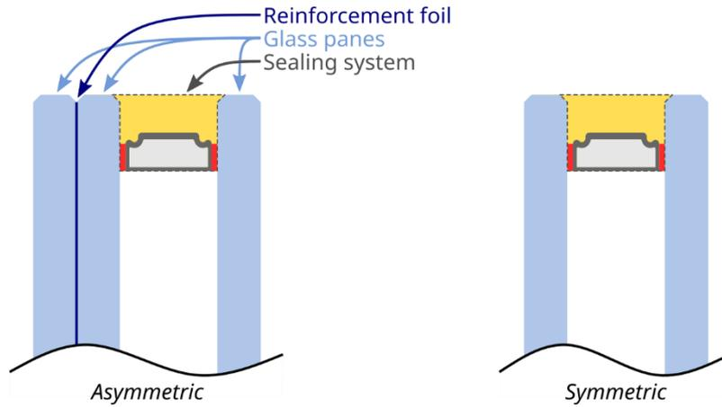
Figure 1: Assembly of the asymmetric and symmetric samples.
