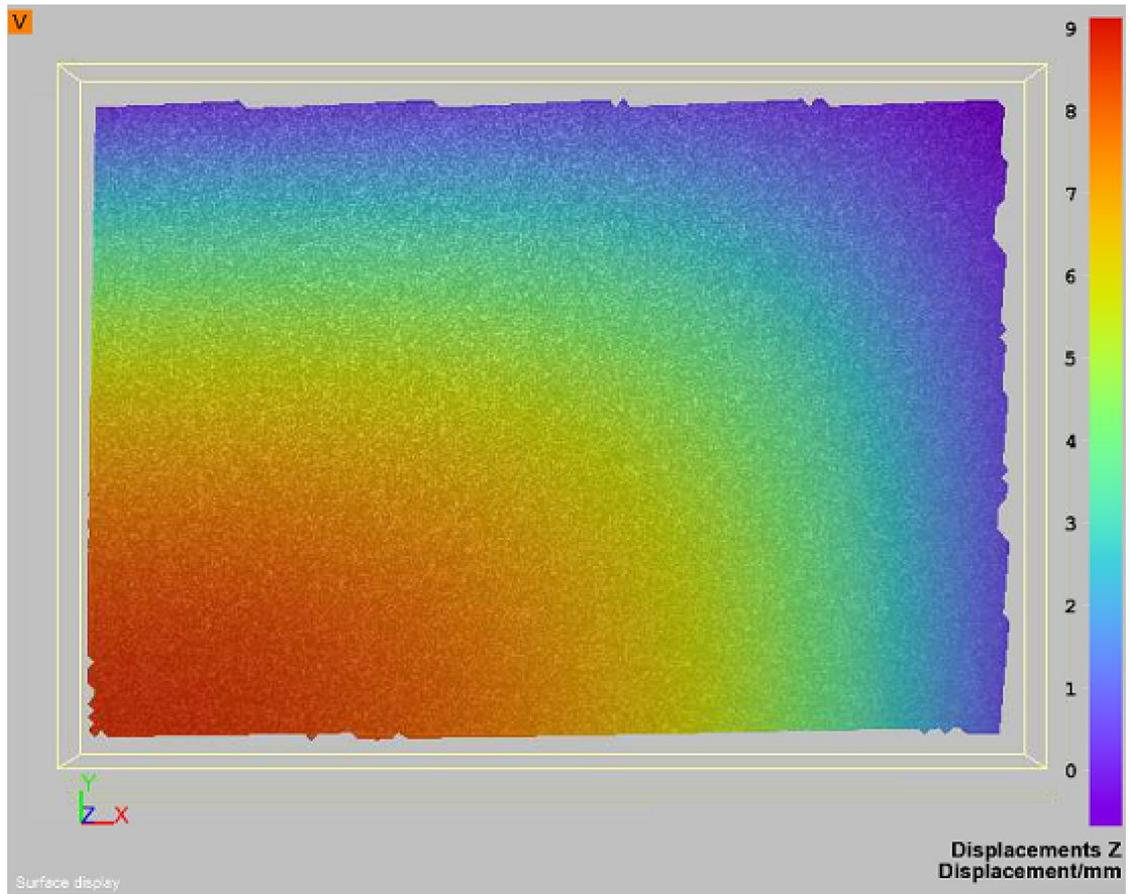
Figure 12: Displacement of sample F at 250 mbar pressure.
