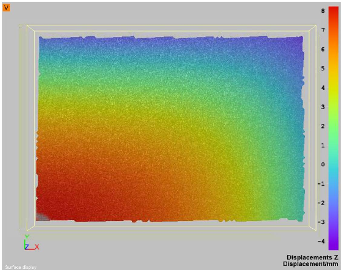
Figure 13: Displacement of the sample G at 250 mbar pressure.
