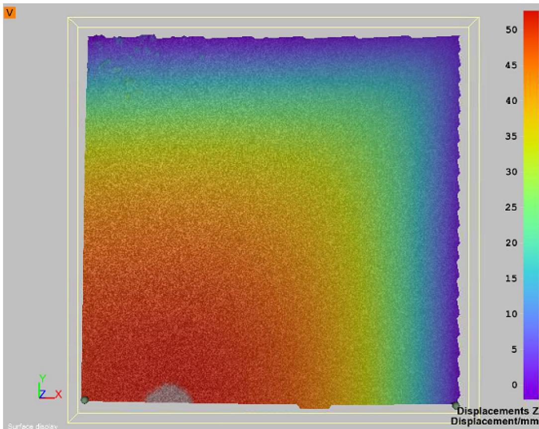
Figure 7: Displacement of sample A at 20 mbar pressure.
