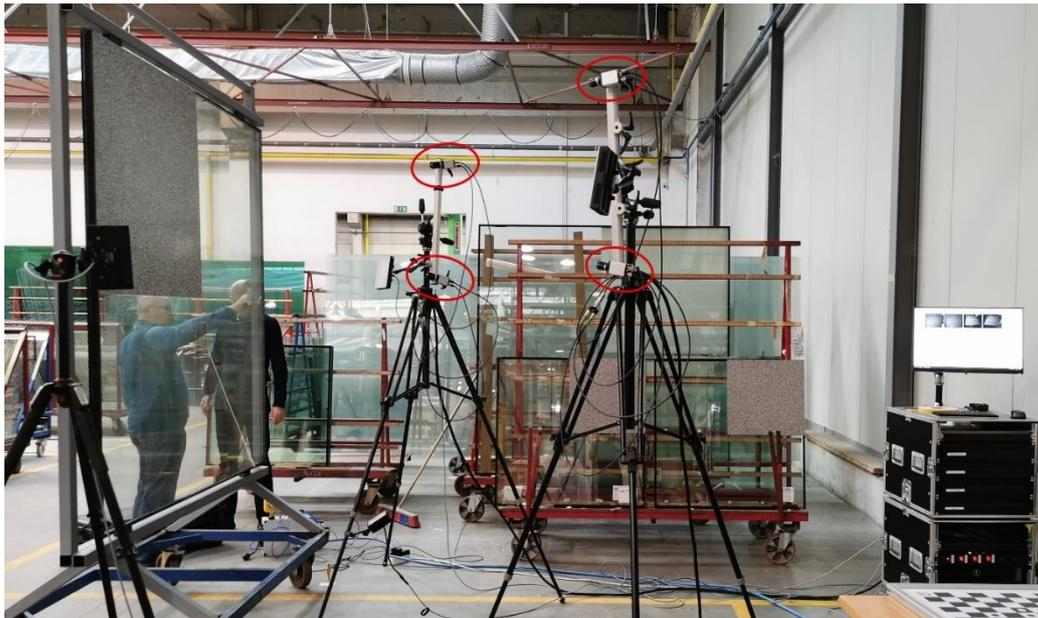
Figure 4: Measurement setup – measurement of displacements of the largest samples. Cameras are circled in red.
